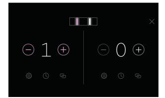
**2.** Press  $\bigcirc$  or  $\oplus$  to adjust the fan speed. There are 5 speeds plus **BOOST**. Press and hold  $\bigcirc$  or  $\oplus$  to jump to 0 or **BOOST**, respectively.
