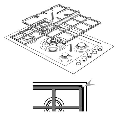
Correct positioning of pan supports
