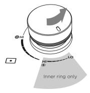
② To use the inner ring of flames only, continue turning the dial towards LO. Only the inner ring will be on in the shaded setting range.
