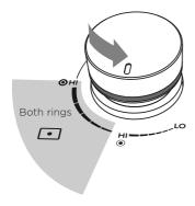
Always start out on HI. Both rings of flame will be on in the shaded setting range.
