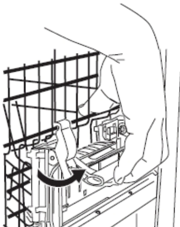
Fig. 7 Adjusting the upper rack for DW60CD models
