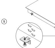
Locate the side brackets\* to the appropriate slots on the cooktop chassis. The correct slot height is determined by the thickness of your countertop.
