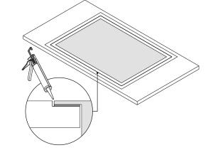
Apply silicone in the gap between benchtop and cooktop Wipe off excess silicone.
