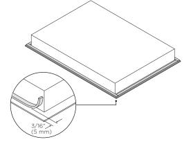
Apply adhesive foam seal around the glass overhang, 3/16" (5mm) from the edge of the glass.
