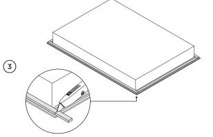
Trim the excess sealing material using a sharp cutter or trimmer knife.
