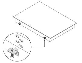
Locate the side brackets\* to the appropriate slots on the cooktop chassis. The correct slot height is determined by the thickness of your countertop.
