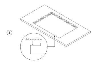
Prepare the countertop for flush installation. Use a router to cut out the edges of the countertop to specified depth 3/16" (5mm). Attach an adhesive tape along
