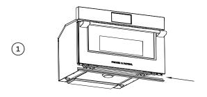
Align the lower trim with the tabs on the base of the oven.
