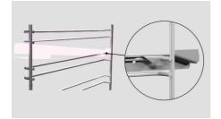
Ensure the rear tags are hooked over the side racks on both sides.
