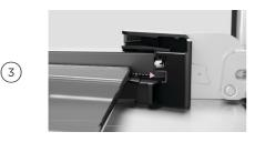
Slide the bottom of the glass into the lower brackets at the bottom of the door.
