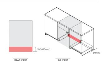
Service outlet at rear extends both sides, hoses and cords can be routed to either or both sides.
