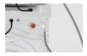
7. Connect the angled end of the short hose (supplied with dryer) to the cold water inlet on the washer.
