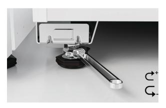
8. With cabinet in the final position, unscrew front levelling feet using the provided spanner. Re-check clearances and alignment before tightening the locking nuts up to the base of the cabinet to lock the feet into position.
