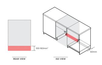
Service outlet at rear extends both sides, hoses and cords can be routed to either or both sides. \*Depending on adjustment of levelling feet.
