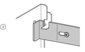
Place chimney around the range hood chassis and hang off the chimney bracket.
