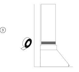
Attach ducting to the ducting adapter using aluminium duct tape.
