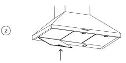
Attach the lower range hood mounting screws to fix the range hood to the wall. Refit the filters.
