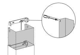
Extend the upper chimney and attach to the upper chimney bracket with 10mm screws.
