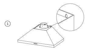
Hang the range hood off the upper range hood mounting screws with 1/16" (2mm) gap. Hang off the keyhole attachment points on the back of the range hood then tighten the screws.
