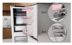
Open the door and remove the door shelves. Unclip hinge covers from middle hinges. Loosen the hinge screws using the supplied Torx T25 driver. Slide the door out and place onto a protected surface.
