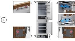
Open the door and secure following the sequence shown. The longer screws should be used where shown in blue, and the smaller screws where shown in red. Ensure a gap between drill and product is maintained to avoid cosmetic damage.
