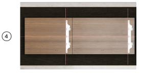
Align the centre door panel bracket to panel ensuring the 'V' in bracket is to sit on the centreline.
