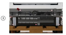
Push the grille flap to open and unscrew the two screws behind the flap and five on the grille. Set screws aside. Open the door and pull the grille outwards from the product.
