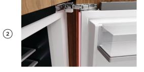
Locate the shorter door trim to the hinge-side of the product, and slide down to clip in place. If a gap is present, remove and readjust the side brackets. Repeat for lower door.
