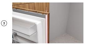
Locate the longer door trim to the nonhinge-side of the product and slide down to clip in place. If a gap is present, remove and readjust the side brackets. Ensure trim does not protrude above the top cover. Repeat for lower door.
