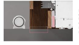
Push the toe kick back to the desired depth before removing. If toe kick depth is less than 3 9/16" (90mm), attach the additional foam block.
