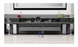
Open the cover and align the grille to the product. Slot into place starting with the base of the grille. Hand tighten the top left screw first, followed by the top right screw. Fit the remaining five screws on the grille to secure.
