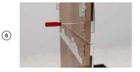
Secure the handle to the panels using 4xM5x25 hex screws per handle. Ensure handle fixings do not interfere with side brackets.
