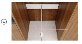
If required, install a spacer at the rear of the cavity to bring depth to 24" (610mm).
