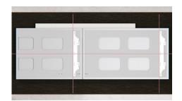
Align the centre bracket to pre-drilled holes on the panel.
