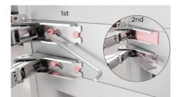
Refit both centre hinge covers by aligning to the hinge as shown, and sliding across to clip back hinge covers into position.
