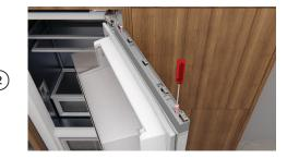
Remove both top covers using a powered driver. Set aside.
