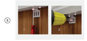
Open the door and loosen the lower bracket screw. Adjust the bracket until it rests against the door panel. Re-tighten the screw and fit an additional screw to secure to panel.
