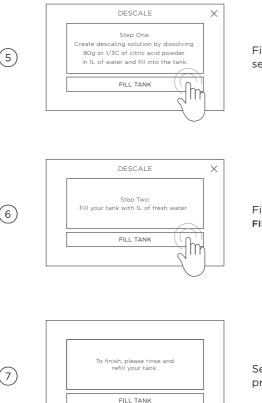
Fill tank with 1L of descaling solution\* and select FILL TANK to begin process.
