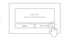
Fill tank with 1L of fresh water and select **FILL TANK** to begin.
