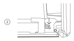
Ensure the door is firmly in place on the hinges. Open the door fully again and push each locking lever down to lock the door onto the hinge.
