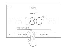
Touch **OPTIONS** at the bottom of the screen and select either: **DELAYED COOK**, **AUTO OFF** and **TEMPERATURE SENSOR**.
