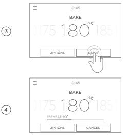
To adjust the preset temperature, swipe left or right or use the dial. Touch **START** to heat the oven and begin cooking.
