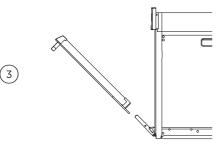
Holding the door on both sides, lift door back up to  $45^{\circ}$  and carefully pull the door out and away from the hinges.
