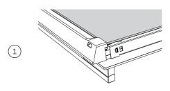
Push the glass retainer tabs in on both sides of the door again. The glass retainer can then be pulled off completely. Gently pull the middle pane toward the top of the door until the pane is clear of the notch at the bottom of the door.
