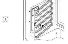
Unscrew and remove the fixing nut at the front of the side rack. Use a coin to loosen the nut if necessary.
