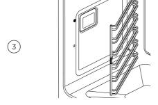
Slide the side rack forward until the rear prongs are clear of the holes.
