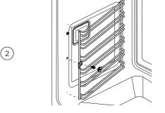
Fit the side rack front tab over the fixing screw.
