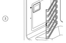
Slide the side rack forward until the rear tabs are clear of the mounting studs.
