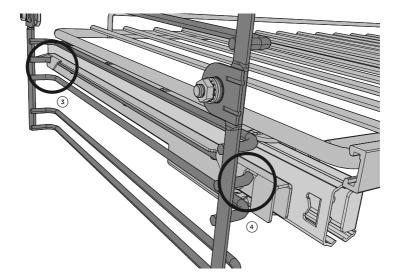
3 Hook the rear tags over the wires of the desired shelf position on both side racks.
