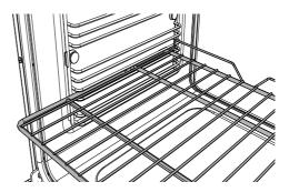
② Position the shelf: it should rest on the side rack wires, as shown.
