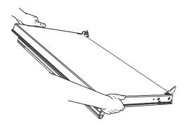
① Hold the door firmly in an approximately halfway open position.
