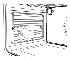
2 Refit the fixing screws and tighten.
