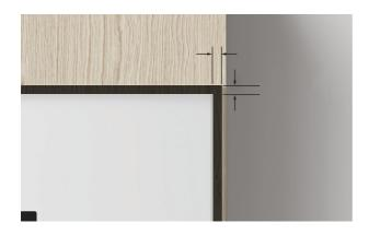
**4.** Check final alignment and ensure required clearances are maintained.
