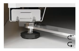
2. With cabinet in the final position, unscrew front levelling feet using the provided spanner. Re-check clearances and alignment before tightening the locking nuts up to the base of the cabinet to lock the feet into position.
