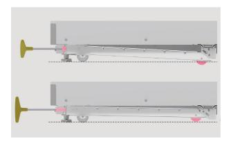
**5.** Lower the rear wheel to achieve clearance between rear feet and floor.
