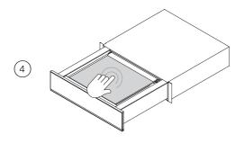
Before pressing the play button  $\triangleright$ , hold down the lid so the gasket forms a seal with the product.
