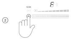
Press and hold  $\circledast$  to clear the alert. If FILTER is still illuminated, ensure the grease filter has been cleaned and refitted correctly
