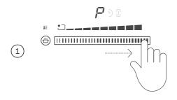
Slide the extraction setting selector to the highest level. Hold until  ${\cal P}$  is displayed.
