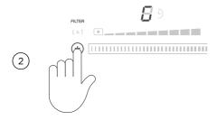
Press and hold  $\circledast$  until FILTER illuminates dimly and  $\Xi$  shows in the display.
