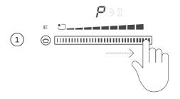
Slide the setting selector to set the cooking zone to the highest heat level. Hold until P displayed.
