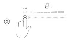
Press and hold \* until FILTER illuminates dimly and  $\textcircled{$\Box}$  shows in the display. Press \* again until F illuminates.
