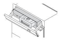
When prompted, press the touch screen to open the control panel. Pull water tank out and fill to the MAX fill line.
