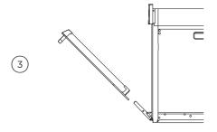
Holding the door on both sides, lift door back up to  $45^{\circ}$  and carefully pull the door out and away from the hinges.
