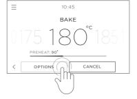
Touch **OPTIONS** at the bottom of the screen and select either: **DELAYED COOK**, **AUTO OFF** and **TEMPERATURE SENSOR**.
