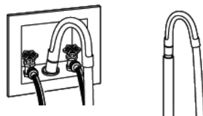
Installing the drain hose
