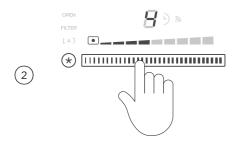
Select an extraction setting by touching or sliding the extraction speed selector with your finger.
