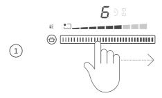
With cooking zone turned on, touch and slide the setting selector to the desired level of reduced heat for the cooking zone.
