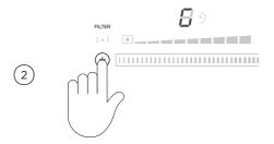
Press and hold \* until FILTER illuminates dimly and £ shows in the display.
