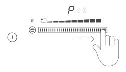
Slide the extraction setting selector to the highest level. Hold until P is displayed.
