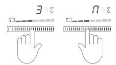
Touch the setting selectors of both bridged cooking zones at the same time. The bridging indicator lights will dim.
