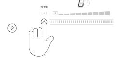
Press and hold  $\circledast$  to clear the alert. If FILTER is still illuminated, ensure the grease filter has been cleaned and refitted correctly
