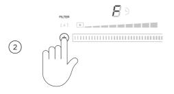
Press and hold \* until FILTER illuminates dimly and  $\textcircled{$\Box$}$  shows in the display. Press \* again until F illuminates.
