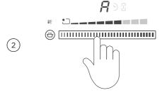
Hold your finger on the selector for 3 seconds until the letter  $\overline{A}$  starts to flash alternately with the selected temperature.
