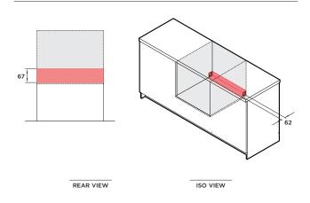
Service outlet at rear extends both sides, hoses and cords can be routed to either or both sides
