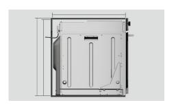
Measure cavity dimensions. Ensure all minimum specifications have been met. Refer to page 6.
