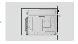
Ensure cavity ventilation has been set up correctly. Refer to page 7 for details.
