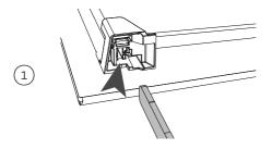
Holding the door on both sides, line up the holes in the base of the door with the hinges and slide the door on.
