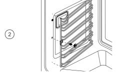
Unscrew and remove the fixing nut at the front of the side rack. Use a coin to loosen the nut if necessary.
