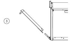
Holding the door on both sides, lift door back up to 45° and carefully pull the door out and away from the hinges.
