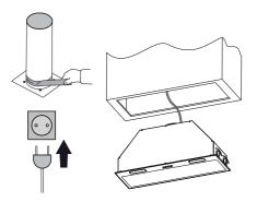
6 Lift the rangehood and fit through the opening of the cupboard till the spring loaded brackets / clips hold the product in place.
