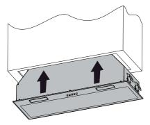
7 Secure rangehood while tightening the brackets / clips.
