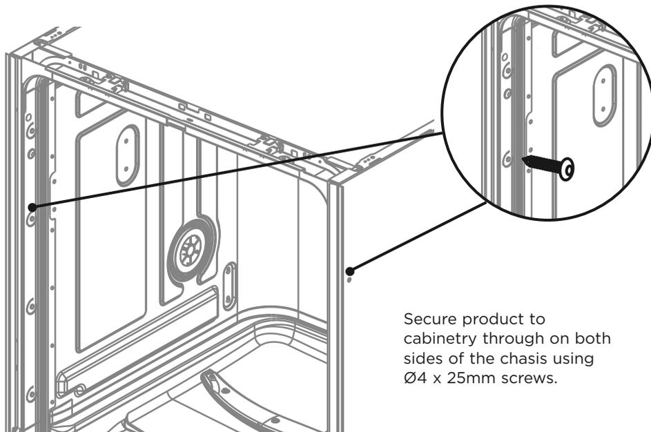
Secure product to cabinetry through on both sides of the chasis using Ø4 x 25mm screws.
