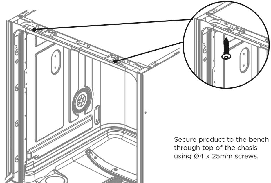
Secure product to the bench through top of the chasis using Ø4 x 25mm screws.
