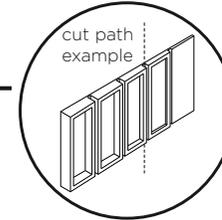
Plastic spacers can be cut to size then taped to the sides of the dishwasher to improve overall stability.
