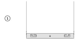
Align the bracket to the chassis ensuring the arrow is facing forward and firmly slot the tabs into place to secure.
