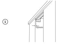
Align the supplied moisture protection tape to the cabinetry as illustrated
