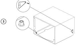
Secure to cabinetry via all three fixing locations in the tub.
