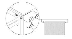
Secure to cabinetry via the brackets. Pre-drilling a pilot hole may be required depending on the cabinetry material.
