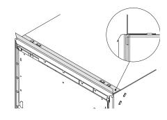
Check the trim seal is facing forward and sitting flat under the bracket.
