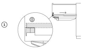
Open the drawer and press both locking tabs back to release.
