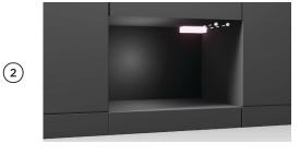
Install the anti-tip block into the cabinetry 14 13/16" (377mm) above cabinetry floor level. Ensure the screws are fitted into wood or metal for stability.
