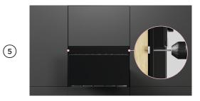
Secure the drawer using the four 7/8" (22mm) screws supplied.
