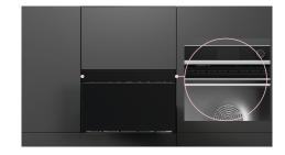
Open the drawer. Using the four holes on the drawer as a template, pre-drill the cabinet using a 1/16" (1.6mm) drill bit.
