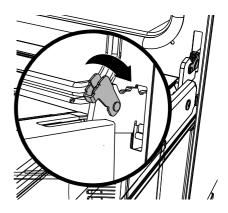
④ Fully close the levers on the left and right hinges, as shown, then close the door.
