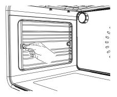
Refit the fixing screws and tighten.
