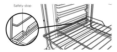
③ Tilt the front up slightly to help the safety stops clear the side rack wires.
