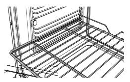
Position the shelf: it should rest on the side rack wires, as shown.
