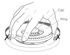
Incorrect and correct positioning of cap and ring – triple-ring wok and dual burner
