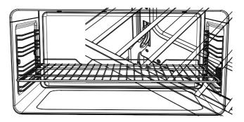
④ Lower the shelf back onto the side rack wires and slide all the way into the oven.
