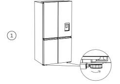
Wind up the feet and carefully ease the refrigerator out of its position. Switch off and unplug.
