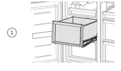
Extend the runners out from the refrigerator. Place the bin on top of the runners.
