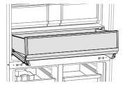
Extend the runners out from the refrigerator. Place the bin on top of the runners.
