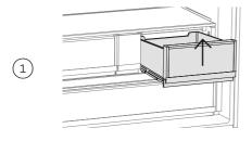
Remove food from the bin. Lift the bin up at the front and pull out over the ledge.
