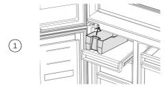
Pull out the tray. Tilt the front of the ice bin up to remove.
