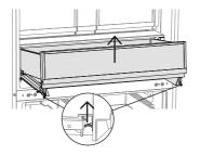
At the same time, on the left and right hand sides push the clip up and lift the bin to release.
