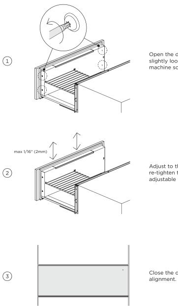
Open the drawer fully, and slightly loosen the T20 star head machine screws.
