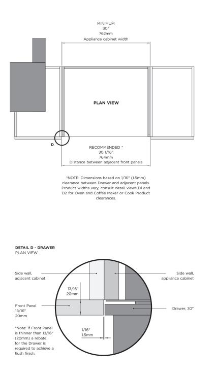
INSTALLATION DETAILS - PLAN VIEW 30" Professional Triple Stack
