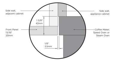
DETAIL D2 - OVEN with rebate PLAN VIEW
