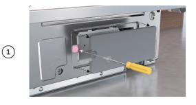
Unscrew and remove the junction box cover to access the terminal block. Do not remove the screw holding the junction box bracket in place.
