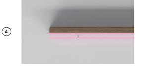
Loosely fit both 16mm Philips hanging screws onto the door panel. Ensure there is a minimum space of 1/8" (3mm) between the screw-head and the panel.
