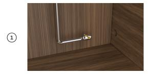
Flush water line into a bucket. Install a hand shut-off valve in a readily accessible location in the adjacent cabinetry.
