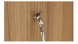
Connect the inlet hose to tap and handtighten into place. Using a spanner or pliers, turn a further 180° to secure. Avoiding over tightening.
