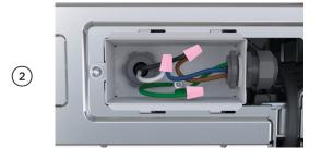
Install the strain relief into the junction box bracket and secure the house wiring or the power cord and tighten. Thread the wires through the hole in the junction box bracket and connect the incoming ground to green, white to white and black to black.
