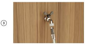
Connect the inlet hose to tap and handtighten into place. Using a spanner or pliers, turn a further 180° to secure. Avoiding over tightening.
