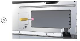
Refit the junction box cover ensuring all wires are clear of the cover. Ensure the power cord is routed under the dishwasher.
