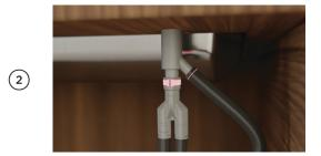
Thread wire clip on to the hose before fitting hose to the supplied hose joiner. Secure using the hose clamps. Fit to the Air Gap Kit. Ensure hose is routed straight to the joiner, remove any excess drain hose.
