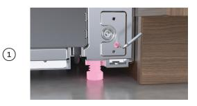
Use a 4mm Allen key to adjust the door tension. Rotate clockwise to increase tension, rotate counterclockwise to decrease tension.
