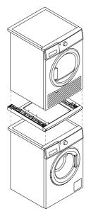
To ensure stacking stability a stacking kit MUST BE USED between the products and fitted correctly to the washing machine and dryer, as per the stacking kit instructions.
