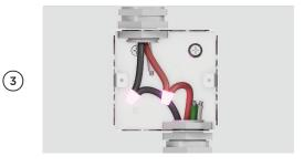
Connect the two black wires together with twist-on connectors and the two red wires together with twist-on connectors.
