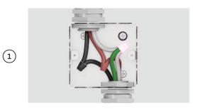
Connect the factory-taped gree and white oven wires to the neutral (white) wire in the junction box.
