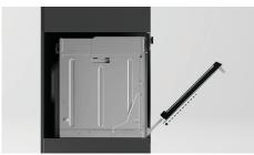
Holding the door on both sides, carefully lift door back onto the hinges.
