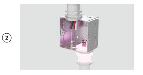
Connect the oven cable to the junction box through the U.L-listed conduit connector.
