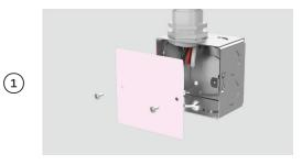
Disconnect the power supply and remove the junction box cover.
