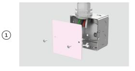
Disconnect the power supply and remove the junction box cover.
