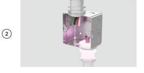
Connect the oven cable to the junction box through the U.L - listed confuit connector.
