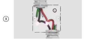
Connect the two black wires together with twist-on connectors and the two red wires together with twist-on connectors.
