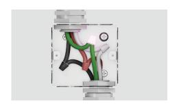
Connect the green grounding oven cable wire to the (green) grounding wire in the junction box. Do not connect the green grounding wire to the neutral (white) wire in junction box.
