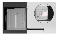
Open the door fully and push each locking lever down and lock into place.
