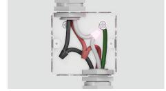
Seperate the factory-taped green and white oven cable wires. If junction box is grounded, connect the green wire to the metal junction box with a screw before connecting the white oven cable wire to the neutral (white) wire in juction box.
