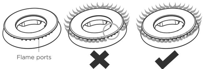
Burner parts may not have been replaced correctly. Check the assembly and make sure the burner cap and/or ring is sitting flat on the flame spreader. See 'Care and cleaning' for illustrations.
