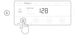
Press and hold for three seconds 1 to select 1/2 LOAD.
