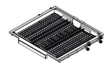
Use the tray to secure cutlery and utensils. Place cutlery into the notches to secure. Place larger utensils in the middle of the tray.
