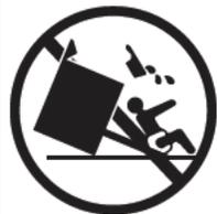
To reduce the risk of tipping the appliance, the appliance must be secured by properly installed anti-tip device packed with the appliance.
