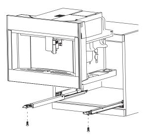
(3) Position the appliance on the rails, making sure the pins are correctly inserted in the housings, then fix it with the screws supplied. If the height of the appliance requires adjusting, use the spacer disks provided.
