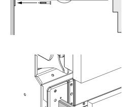
Fix brackets to panel using Ø3.5 x 12mm screws. Insert toe kick into product and mark the desired alignment depth on the bracket.
