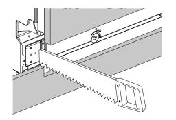
Note door overhang and swing range relative to height and depth of toe kick panel. As the panel is continuous, cutting back panel is likely to be necessary to ensure seamless integration.
