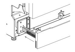
Slide toe kick firmly back into the product to attach. The bent tabs will prevent the toe kick receding into the product further than desired.
