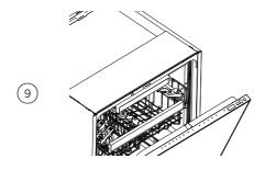
After the wash the door will automatically open slightly to assist with drying.\*
