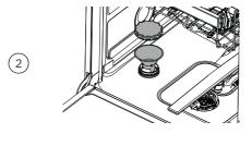
Turn the cover anticlockwise, then pull to remove. Add salt to the reservoir using the funnel provided.
