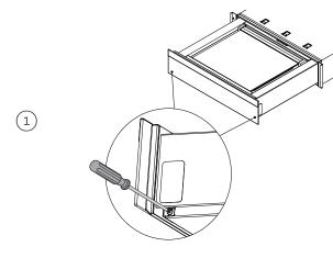
Open the drawer fully, and slightly loosen the two screws.
