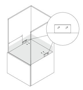
Locate the attachment position of the anti-tip brackets in both sides of the cabinetry,
