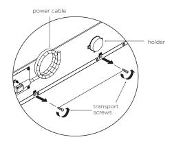
Unscrew the transport screws from under the power cable and holder.
