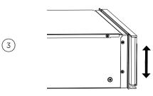
If required, adjust panel vertically as needed.
