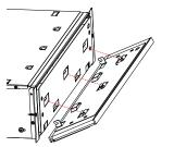
Align the tabs on the panel to the chassis and slot into place.
