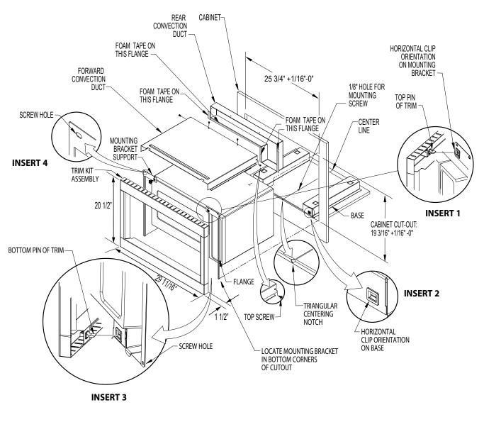
Note: when installed, the trim assembly is positioned symmetrically over the cabinet cut-out
