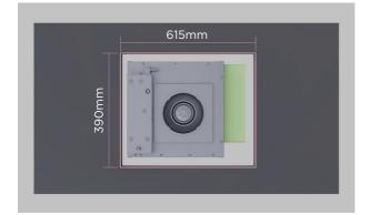
**2.** Create a 615x390mm cutout in the base of the cavity for the external blower.
