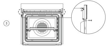
Use the supplied screws to secure the oven to the cabinetry.
