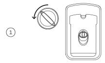
Turn the cap anticlockwise and remove.
