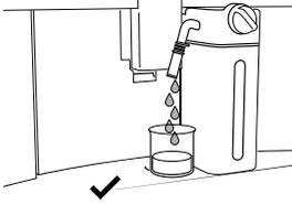
The milk container has been inserted with the froth adjustment dial in the CLEAN position.
