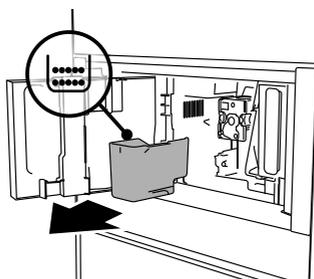
When EMPTY GROUNDS CONTAINER appears on the display, the grounds container must be emptied and cleaned. The appliance cannot be used to again until you have cleaned the grounds container. Even if the container is not full, the empty grounds container message is displayed 72 hours after the first coffee has been prepared. For the 72 hours to be calculated correctly, avoid turning the appliance off from the mains switch if it is not necessary.
