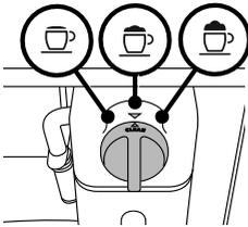
The milk container has been inserted with the froth adjustment dial in the CLEAN position.
