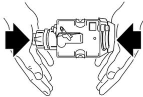
Note: If you encounter difficulty inserting the infuser, before inserting it you must adapt it to the right dimension by pressing it forcefully from the bottom and top as shown.
