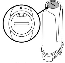
Note: The filter lasts about two months if the appliance is used normally. If the coffee maker is left unused with the filter installed, it will last a maximum of three weeks.
