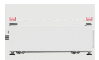
2. Place the plinth in its final install location. Adjust the feet using the supplied spanner until the plinth is level front to back and corner to corner.
