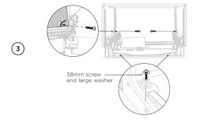
Secure to cabinetry via all three fixing locations in the chassis.
