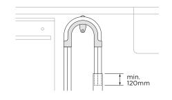
Pull the hose through the support guide and rest in standpipe.
