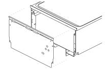
Carefully pull the bracket down and out from DishDrawer™ Dishwasher and unplug the Knock-to-Pause module and earth wire.
