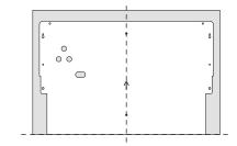
On the back of the panel, mark the centre and align the base of the bracket with the base of the panel.
