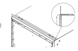
Check the trim seal is facing forward and sitting flat under the bracket.
