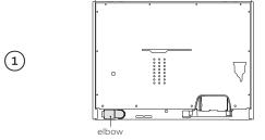
Rotate the elbow at the rear of the product to either the left or right depending on your venting location.
