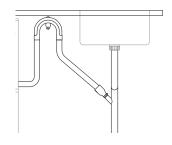
Pull the hose through the drain hose support before threading the wire clip on to the hose and fitting to the supplied hose joiner. Secure using the wire clips.
