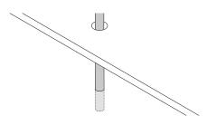
Route the venting hose through the floor. Ensure any excess hose is removed.
