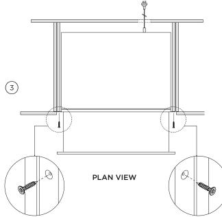
Open the drawer and secure the attachment flanges of the drawer to the side edges of cabinetry with T20 star head machine screws (4x).
