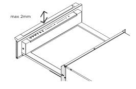
Adjust to the required height and then re-tighten the screws. The height is adjustable within 1/16" (2mm).
