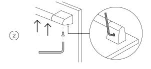
Insert the socket screws and tighten from the base of the handle using the supplied Allen key. Apply upward pressure to the handle while tightening to reduce the risk of damage.
