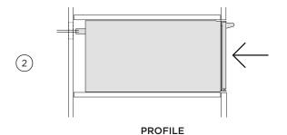
Push the warming drawer back into the cabinetry, and align the front panel with the cabinetry as desired.
