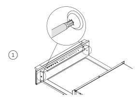
Open the drawer fully, and slightly loosen the screws.
